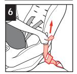
Place one knee in the child restraint and push down firmly while pulling up on loop end of the LATCH belt to tighten.
